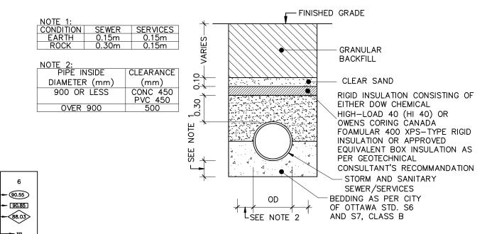
THERMAL INSULATION FOR STORM/SANITARY SERVICES IN SHALLOW TRENCHES
