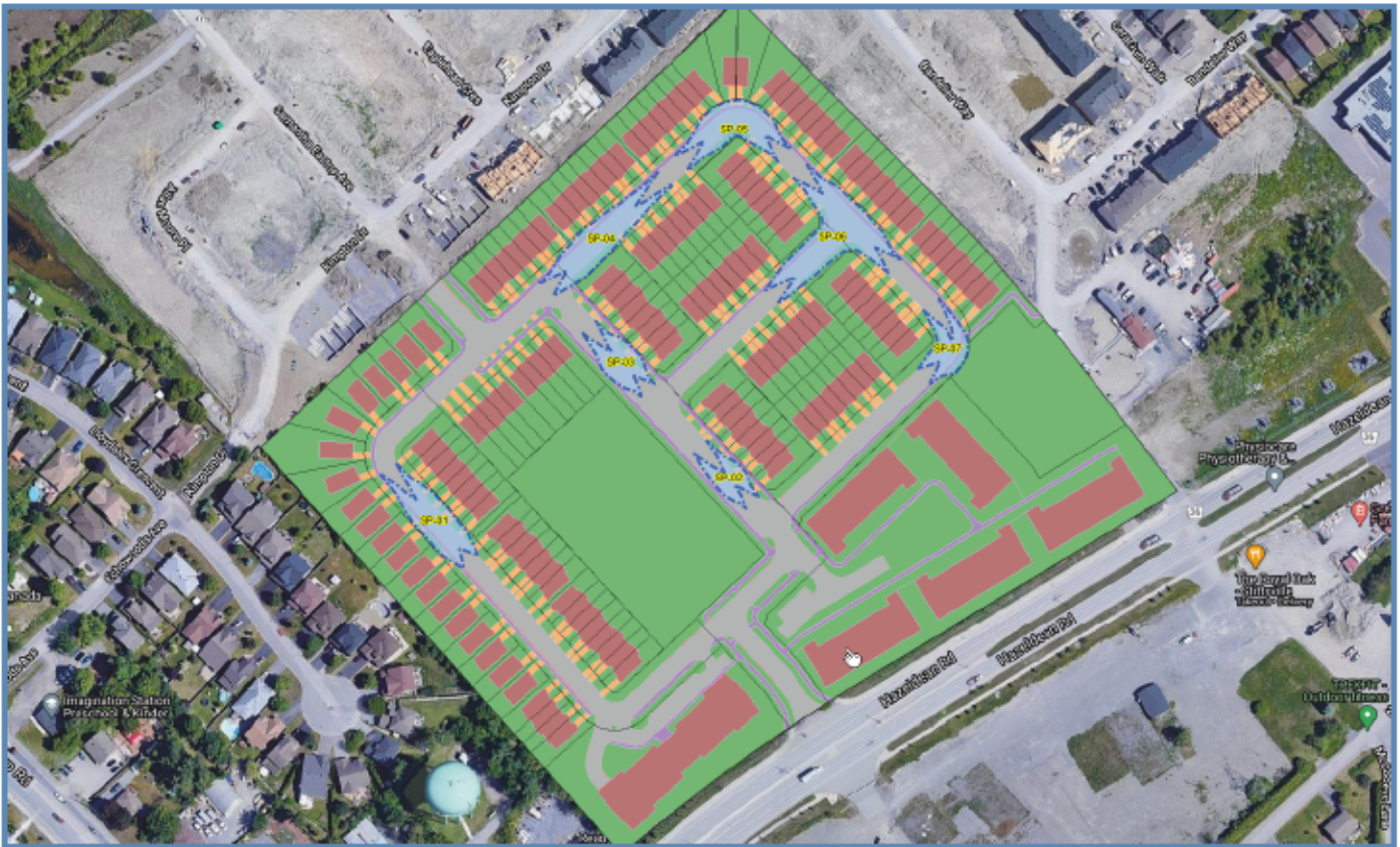
Figure 7-1: Surface Ponding Locations
