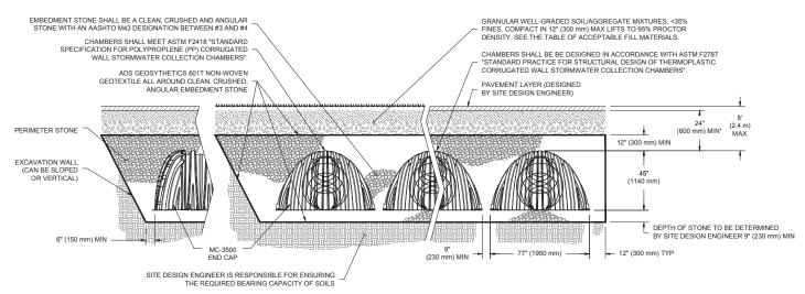
\*MINIMUM COVER TO BOTTOM OF FLEXIBLE PAVEMENT. FOR UNPAVED INSTALLATIONS WHERE RUTTING FROM VEHICLES MAY OCCUR, INCREASE COVER TO 30" (750 mm)
