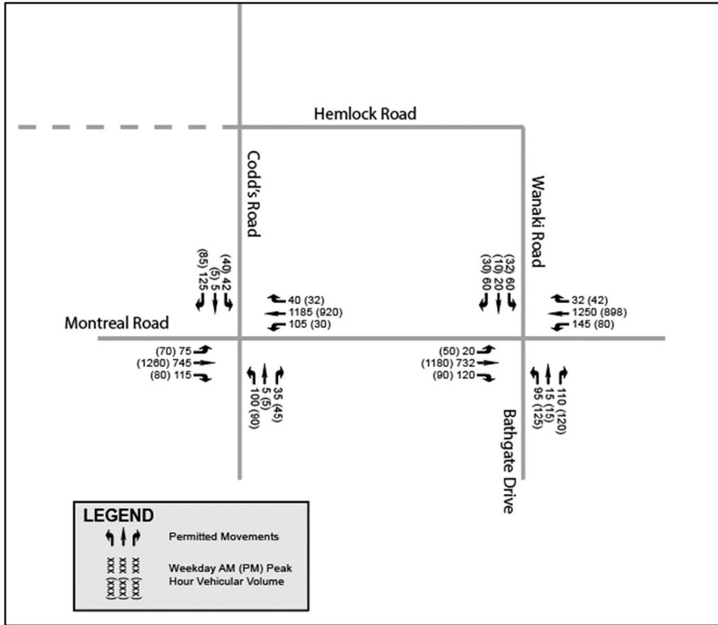
Figure 7 – Existing Lane Configurations and Intersection Control
