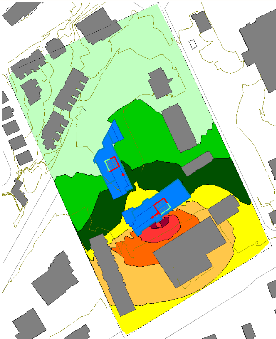
FIGURE 7: GENERATOR NOISE CONTOURS (37.4 M ABOVE GRADE, WITH ACOUSTIC LOUVRE)
