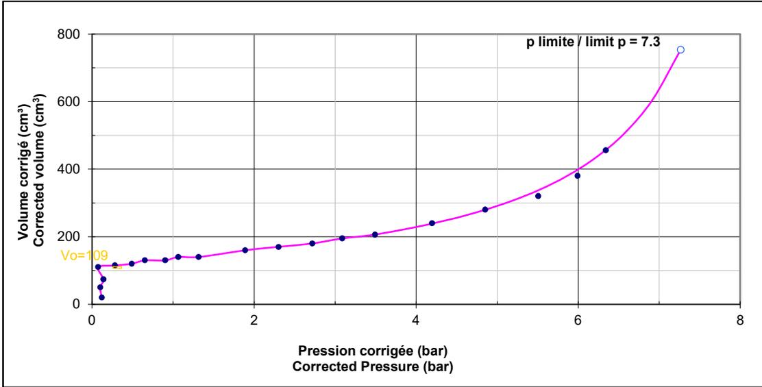
Figure 1: PMT01 curve at 1.5 m depth
