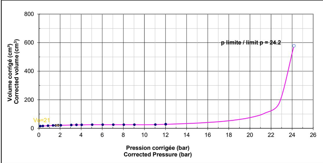
Figure 3: PMT02 curve at 1.2 m depth
