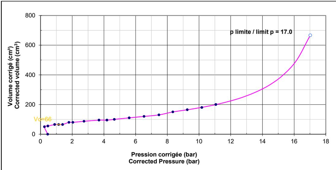
Figure 5: PMT04 curve at 3.0 m depth
