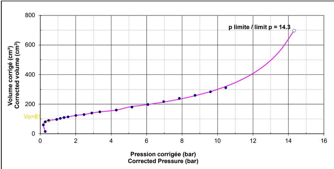
Figure 4: PMT03 curve at 3.0 m depth
