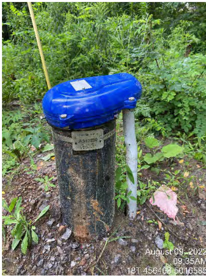
Photo 6 - Observation well (ID A342260) used during pumping test for monitoring of potential interference effects.
