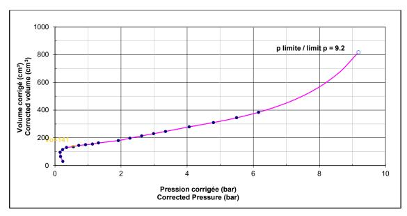
Figure 2: PMT01 curve at 3.5 m depth
