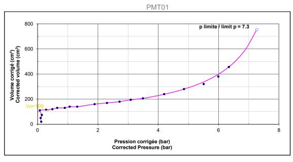
Figure 1: PMT01 curve at 1.5 m depth
