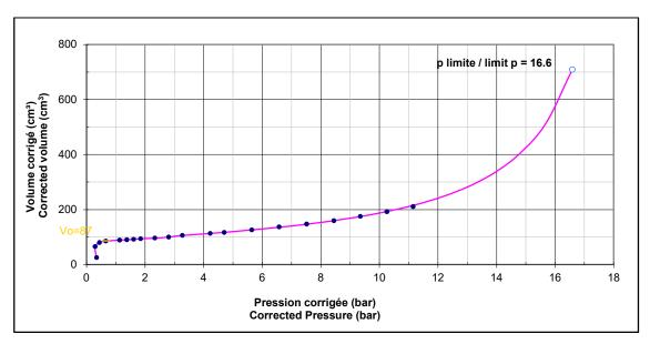
Figure 6: PMT03 curve at 4.5 m depth
