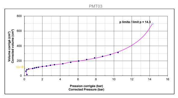
Figure 4: PMT03 curve at 3.0 m depth
