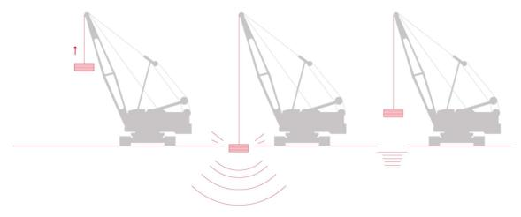
Figure 1 – Dynamic Compaction process
