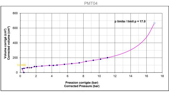
Figure 5: PMT04 curve at 3.0 m depth
