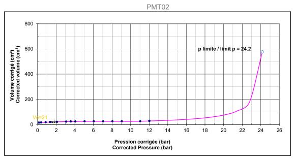
Figure 3: PMT02 curve at 1.2 m depth
