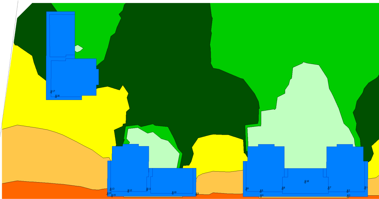
FIGURE 5: NIGHTTIME TRAFFIC NOISE CONTOURS (10 M ABOVE GRADE)
