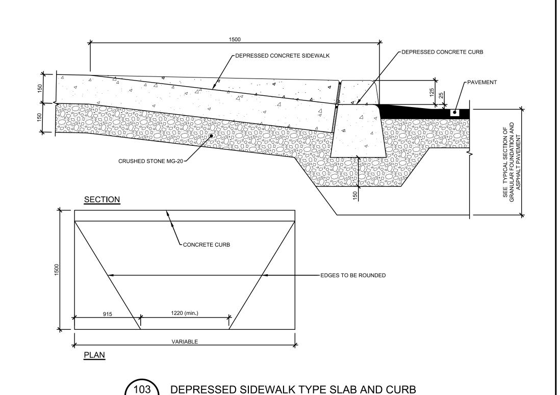
SIDEWALK - BUILDING TYPE - SLAB AND CURB
