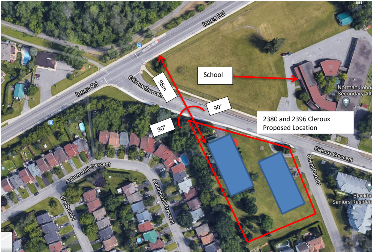
Figure 2.2 – Surrounding area of 2380 and 2396 Cleroux Crescent with locations, distances and angles of relevant noise sources
