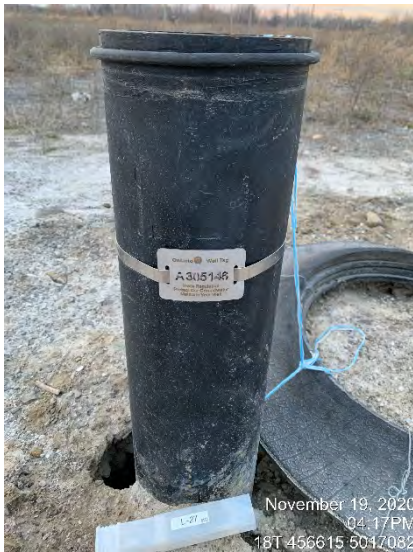
Photo 3 - Example of observation well (ID A305146) used during pumping test for monitoring of potential interference effects.
