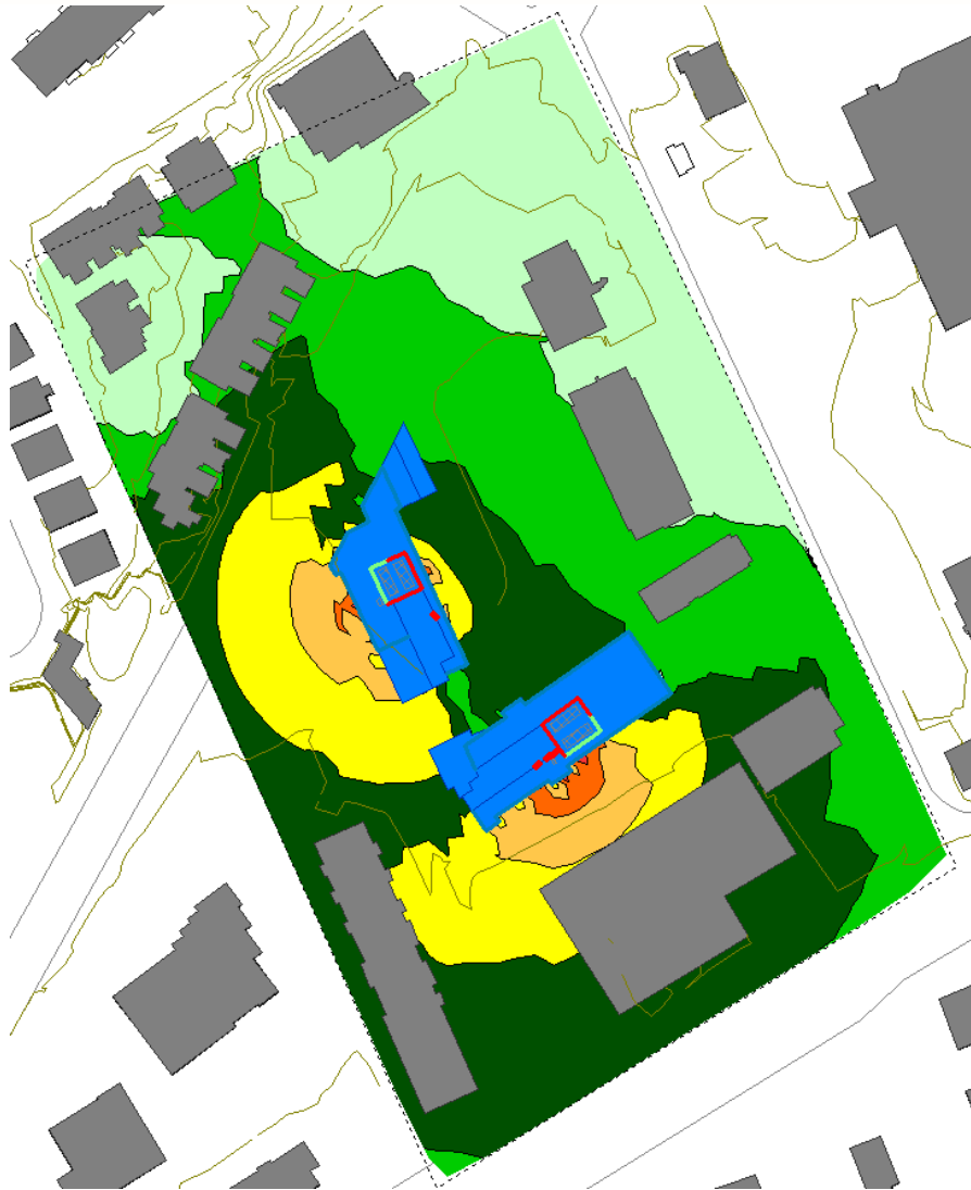
FIGURE 6: HVAC NOISE CONTOURS NIGHTTIME (37.4 M ABOVE GRADE, WITH 4-M NOISE SCREEN AND ACOUSTIC LOUVRE)
