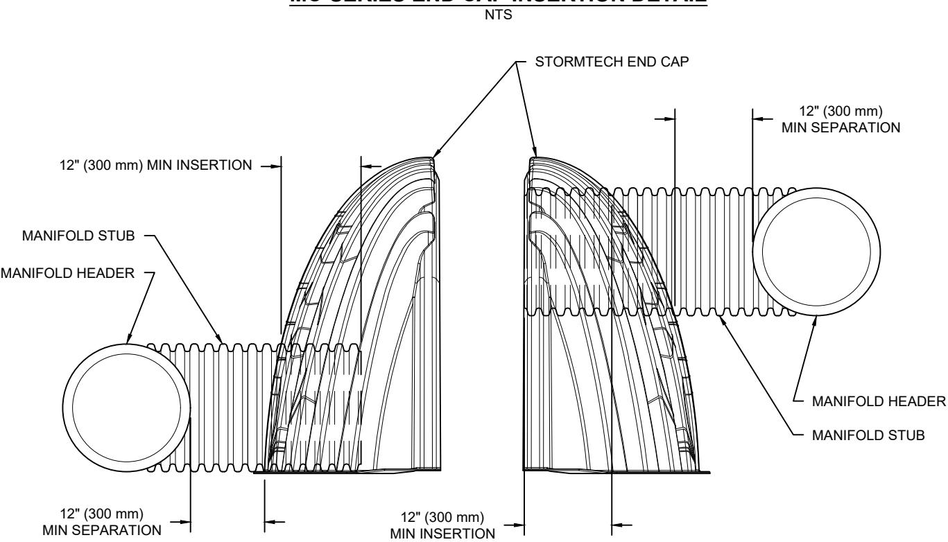
NOTE: MANIFOLD STUB MUST BE LAID HORIZONTAL FOR A PROPER FIT IN END CAP OPENING.
