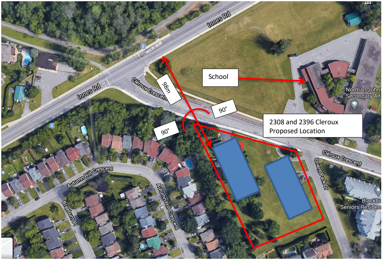
Figure 2.2 – Surrounding area of 2308 and 2396 Cleroux Crescent with locations, distances and angles of relevant noise sources
