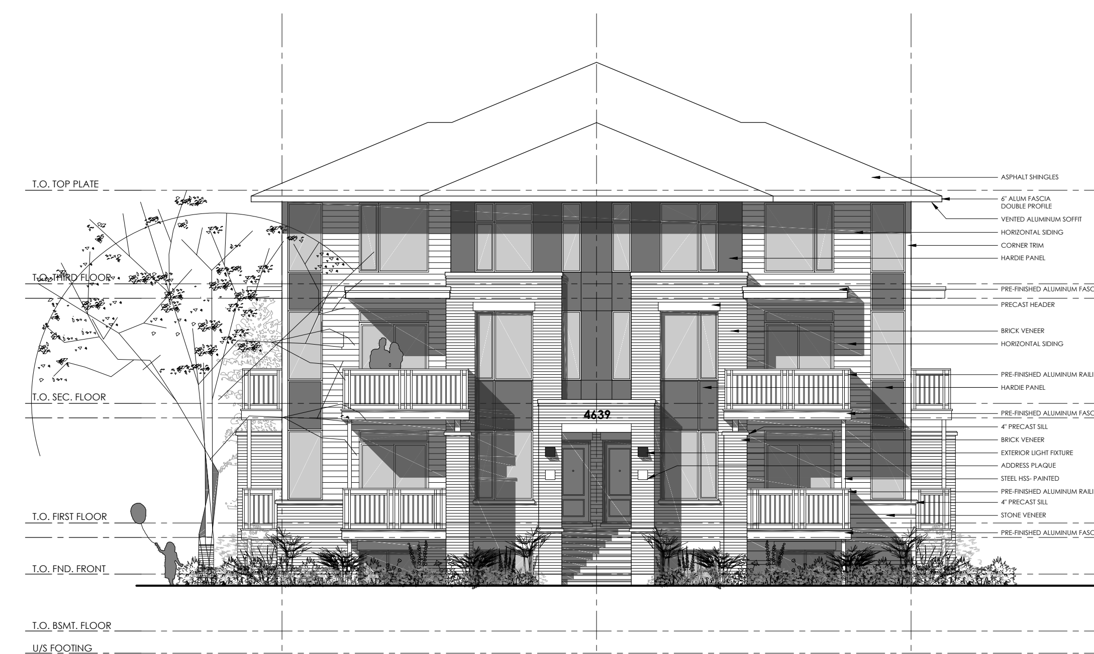
4 EXTERNAL END ELEVATIONS (NORTH & SOUTH) A2 SCALE: 1:100
