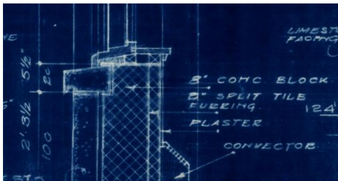
Figure 12; Detail section through the Kent and Gilmour facades illustrating the arrangement of the limestone sill course and limestone cladding. The sills are bonded to the limestone cladding and the concrete back-up wall making it difficult to salvage the window sill course material. The drip edge only adds to the difficulty of successfully salvaging the material for reuse. Source: 1955 Drawing Set A4
