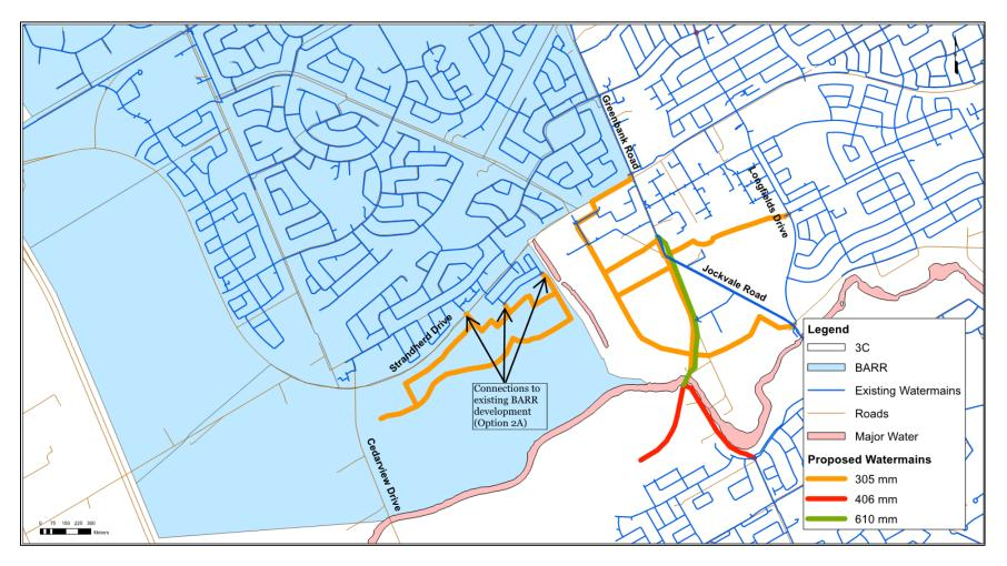
Figure 2-5: Proposed Pipe Layout Post Zone Reconfiguration – Scenario 2A
