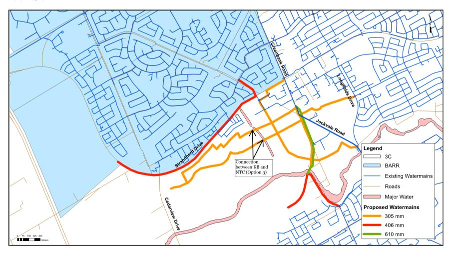
Figure 2-7: Proposed Pipe Layout Post Zone Reconfiguration – Scenario 3
