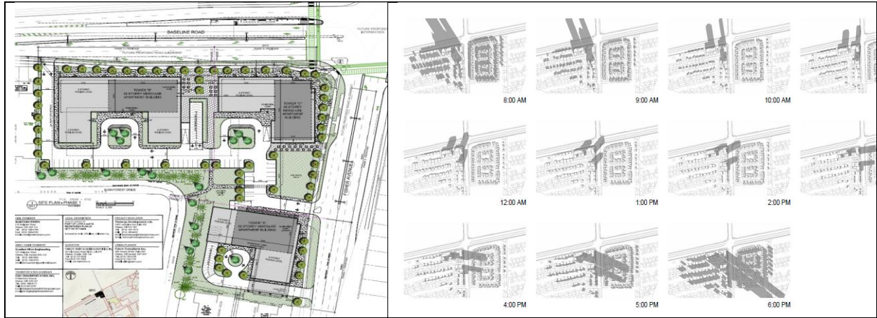
Figure 23: Site Plan and September Solstice Shadow Study illustrating the shadow cast by the three towers with 6 storey podiums and two slab towers along Baseline. Source: Zoning Amendment dated 2022 05 16. Rod Lahey Architects Inc. 2022
