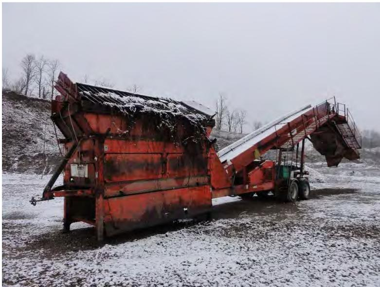
Photo 16 – Sand filter machine (currently inactive) located on the east portion of the Site (no evidence of any stains or spills observed).
