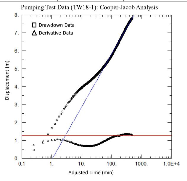
Estimated Hydraulic Conductivity (k) =  $8 \times 10^{-5} \text{ m}^2/\text{s}$  or  $6.8 \text{ m}^2/\text{day}$
