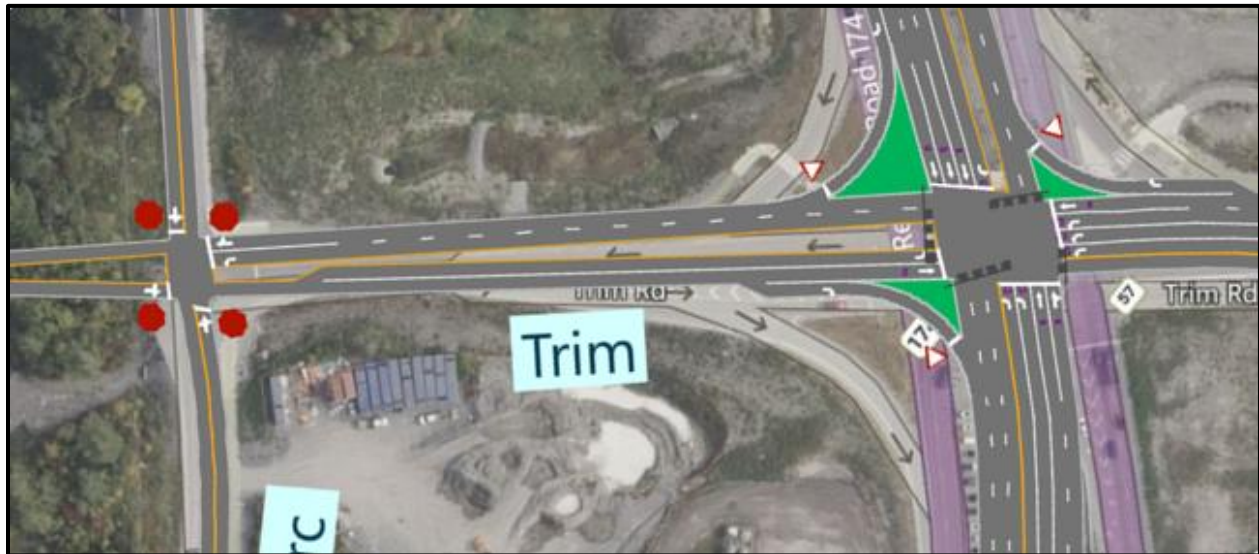
Figure 32: Lane Geometry Modifications Required to Support Scenario 1
