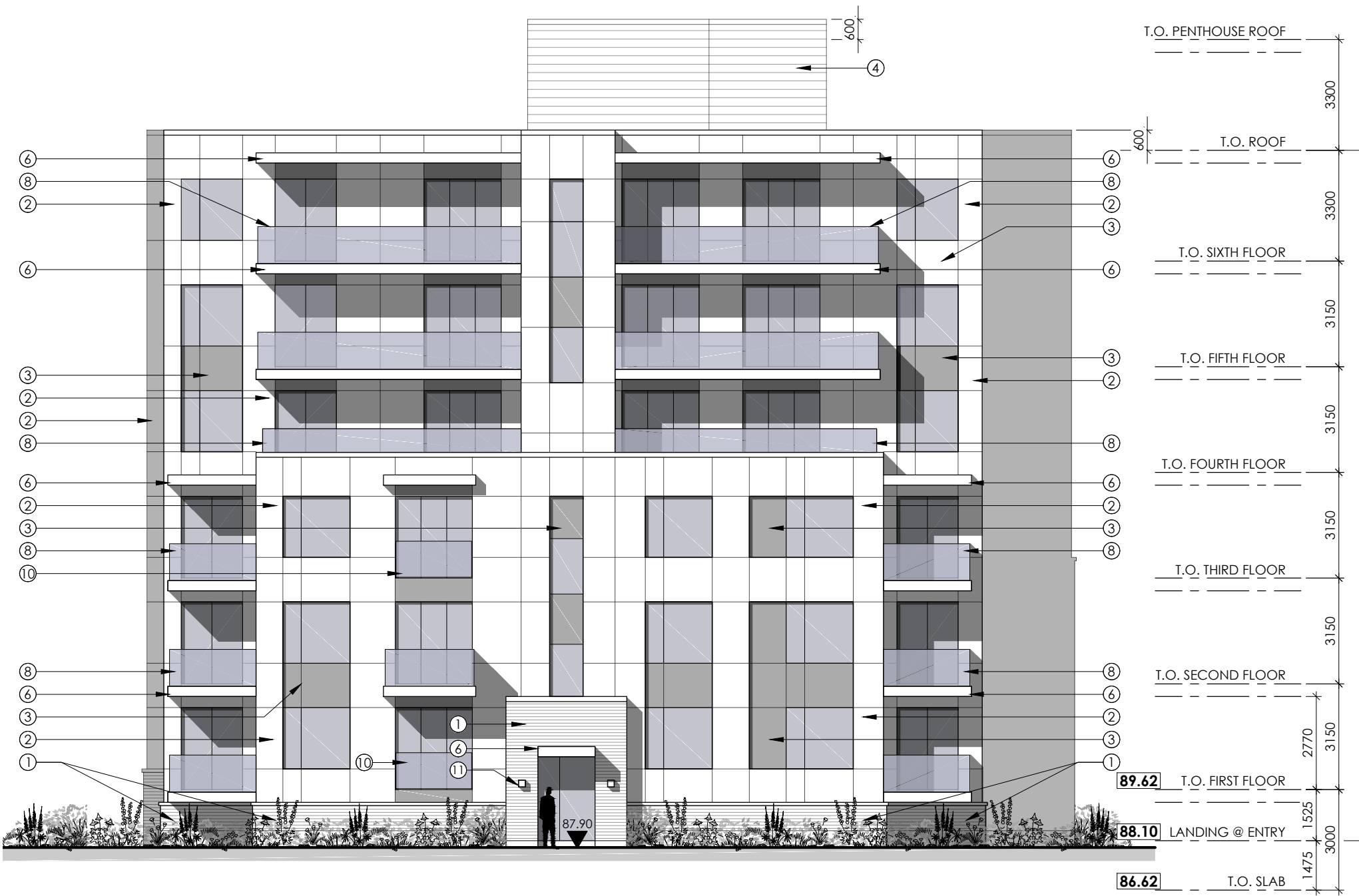
REAR [NORTH] ELEVATION
