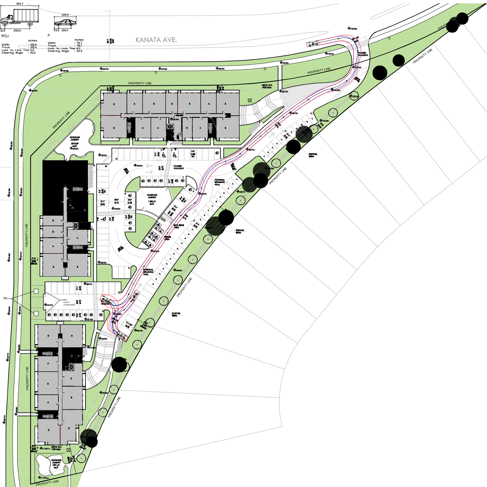
Waste Collection Truck Width : 78.7 Track : 192.4 Lock to Lock Time : 6.0 Steering Angle : 127.7
