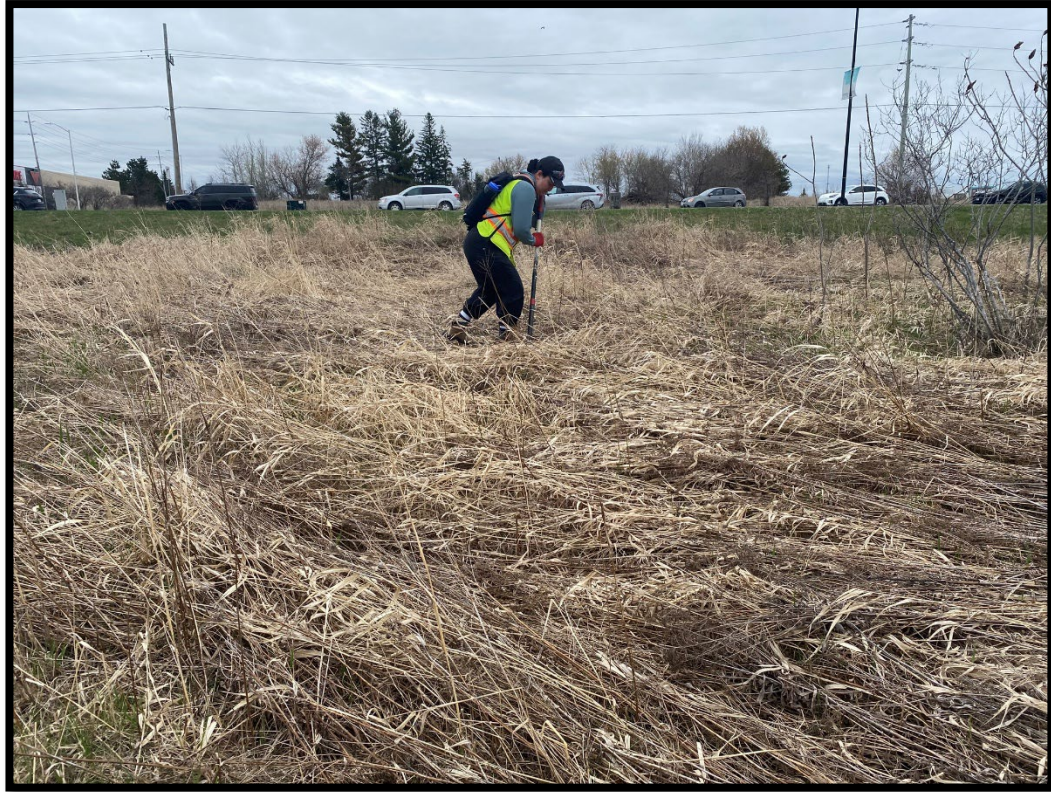
Figure 23: Test pitting in progress (MH1446-D058).
