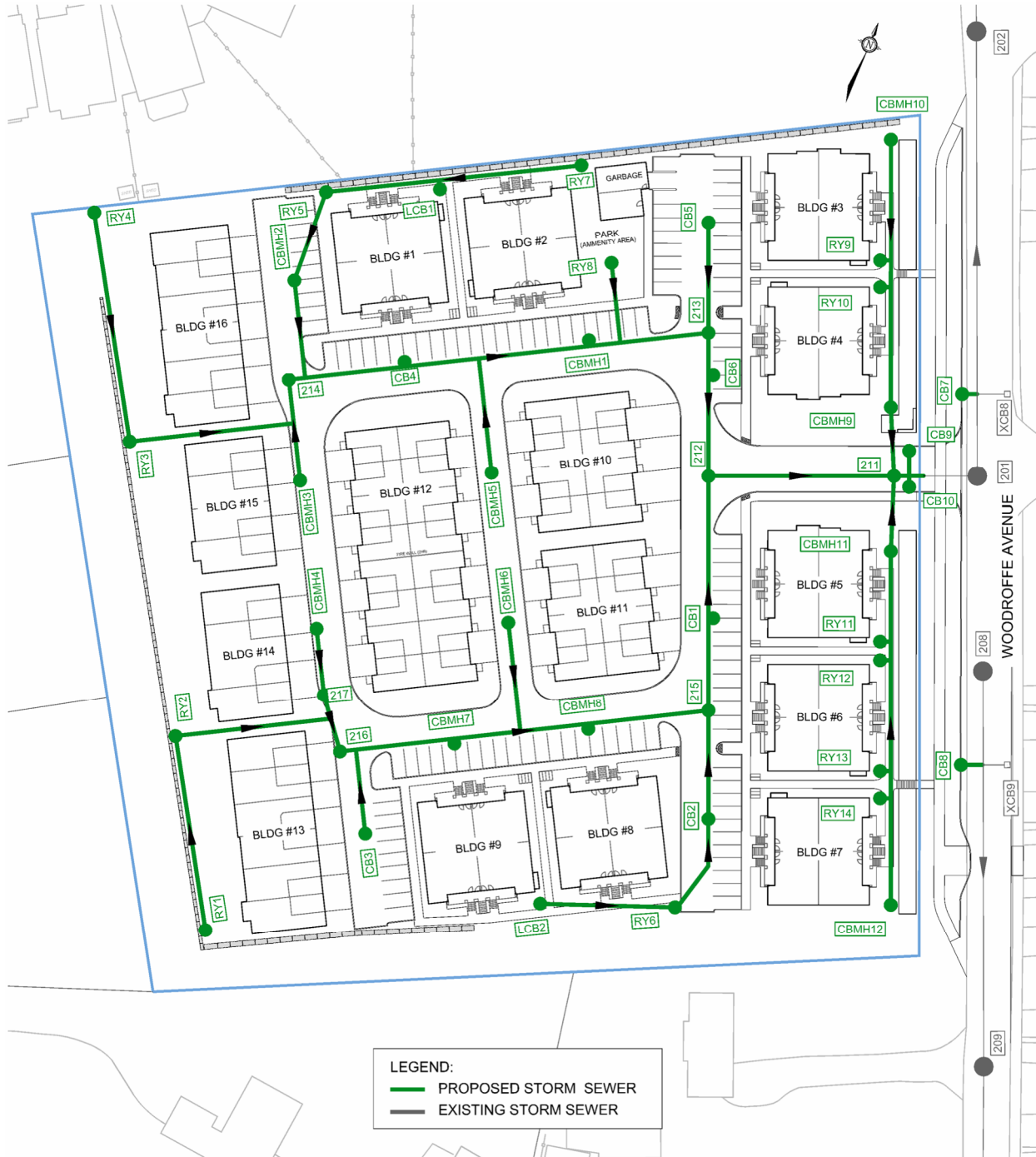
Figure 5: Storm Sewer Network
