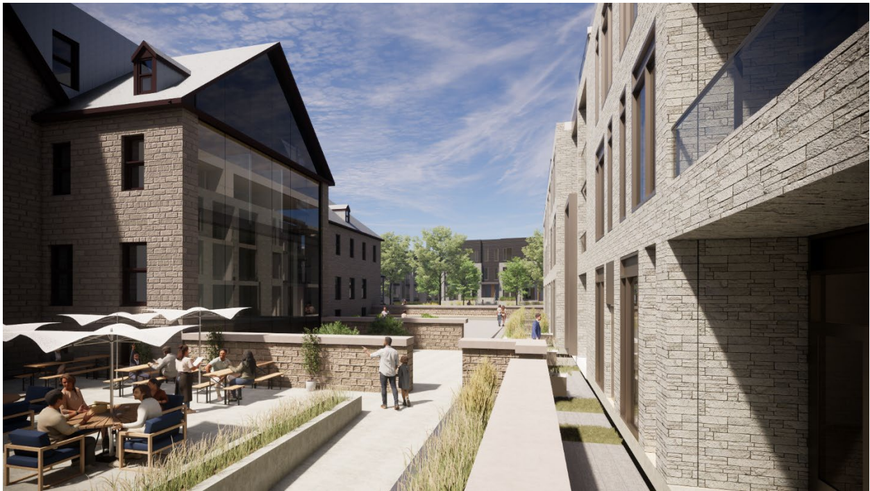
Figure 32: Illustration of the proposed courtyard design with low walls constructed from salvaged stone demarcating the demolished north and south wings, and the alignment of the east elevation of the new apartment building along the former line of the demolished west wing to recreate a sense of enclosure. (Project1 Studio)
