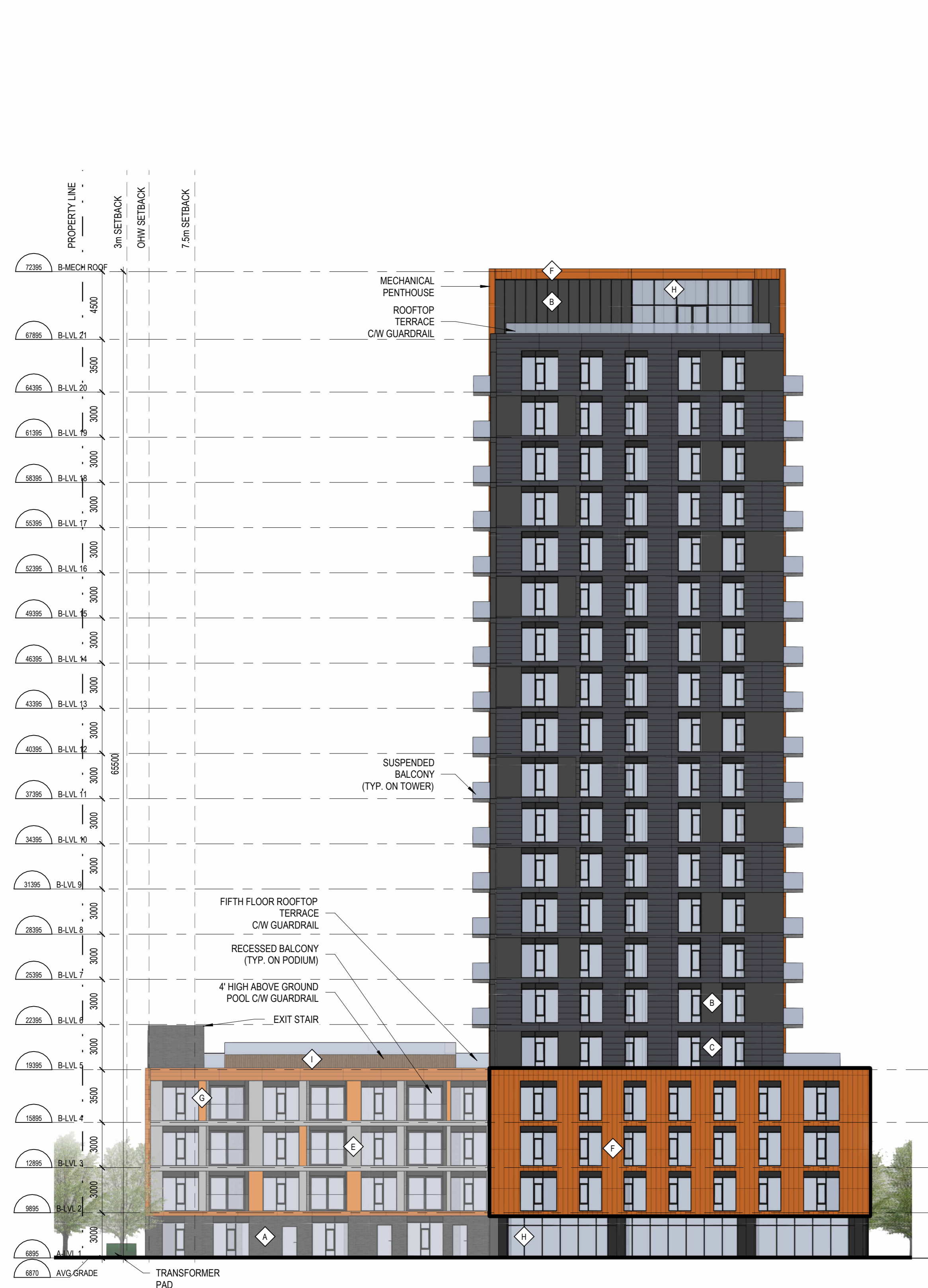
1 NORTH ELEVATION - TOWER B A.202 ÉCHELLE / SCALE: 1:200
