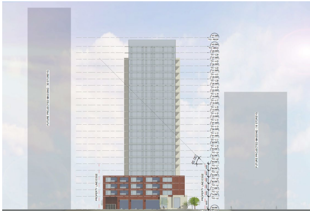
Figure 14: High-projection 45-degree angular plane towards northern properties (Source: RLA Architecture)
