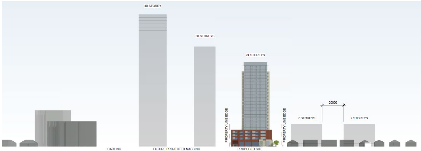
Figure 11: Low-projection massing transition along the west side of Edgeworth Avenue (Source: RLA Architecture)
