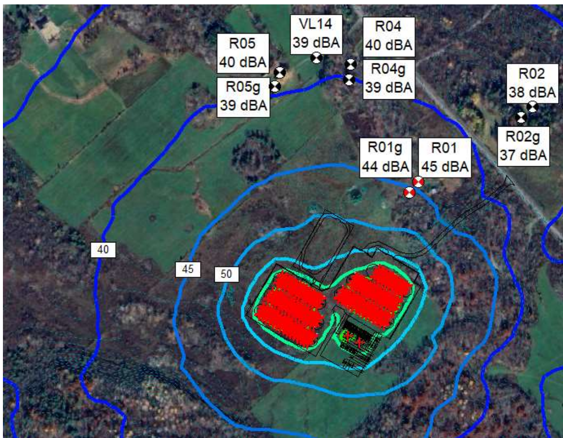
Figure 6: Option 4 – Equipment Sound Level or Tonality Reduction – Noise Contours at 4.5m Height
