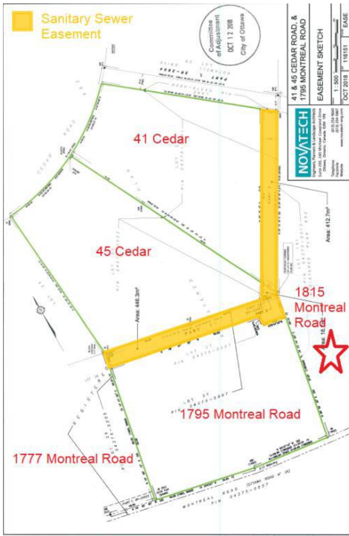
Figure 7: Sanitary sewer easement highlighted, approved by Committee of Adjustment Decisions D08-01-18/B-00369; D08-01-18/B-00370; D08-01-18/B-00368.
