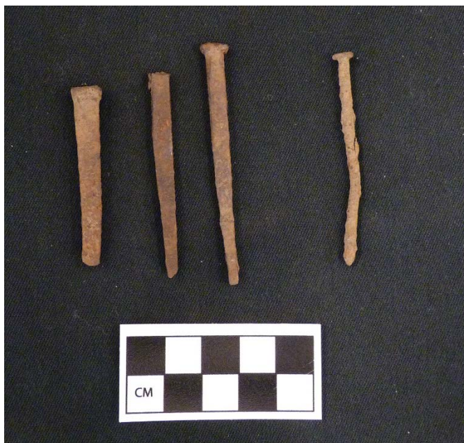
Image 23: Representative sample of nails. The three nails on the left are cut while the last nail on the right is wire.
