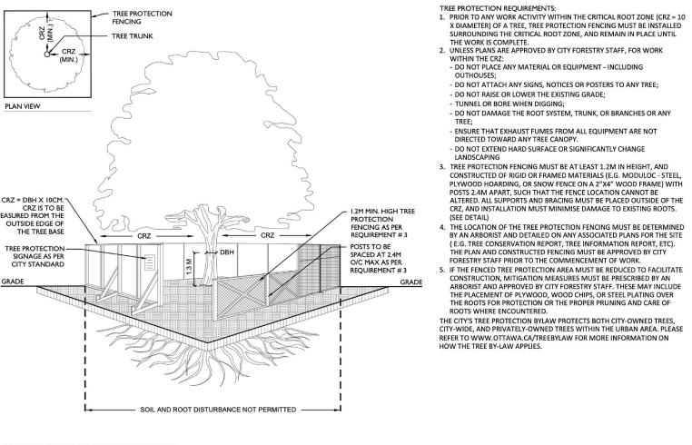
TREE PROTECTION SPECIFICATION TO BE IMPLEMENTED FOR RETAINED TREES, BOTH ON SITE AND ON ADJACENT SITES, PRIOR TO ANY TREE REMOVAL OR SITE WORKS AND MAINTAINED FOR THE DURATION OF WORK
