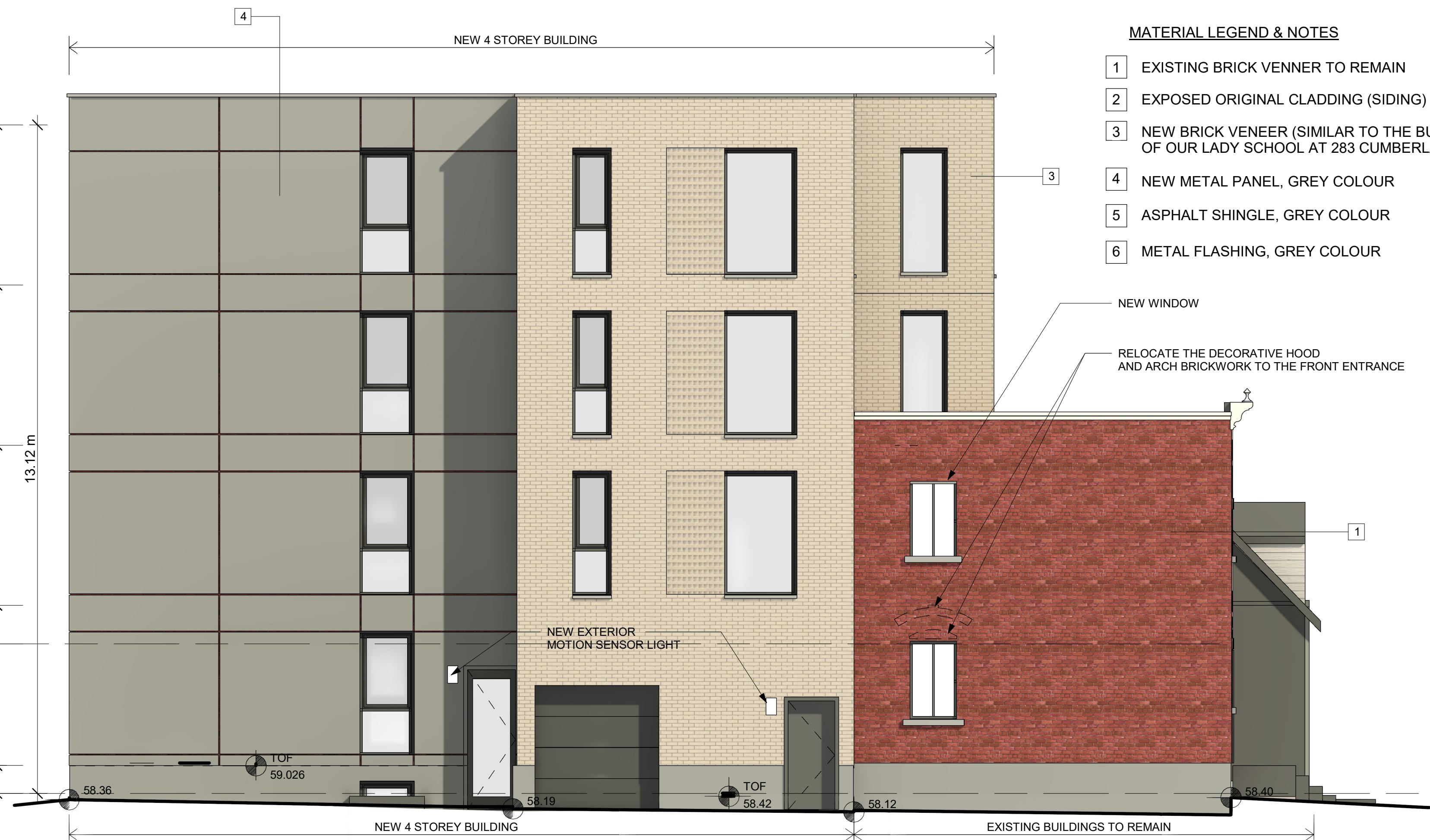
4 Side (East) Elevation 3/16" = 1'-0"
