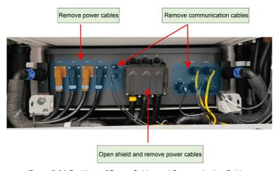
figure 5-31 Positions of Power Cables and Communication Cables
