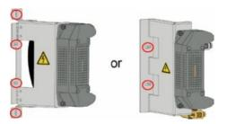
figure 5-13 Fuse mounting holes
