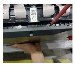
**Step 4** Hold the BMU box with your left hand, pinch both sides of the BMU top cover with your right thumb and forefinger, and then gently remove the BMU with firm force. Since the flexible flat cable (FFC) is partially connected to the BMU box, do not pull it outwards with excessive force.
