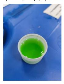
**Step 5** Test the coolant sample with the PH test paper or PH meter to obtain the current coolant PH value. When the value is below 7.3, it is required to change the coolant (drain and refill the system).
