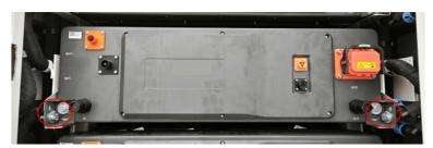
figure 5-14 Positions of M10 Screws
