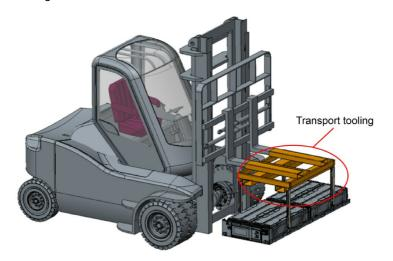
figure 5-6 Transport tooling with forklift schematic
