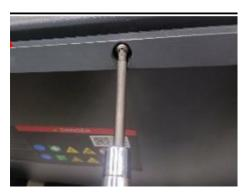
**Step 2** After removing the screws fixing the BMU box, hold the BMU box from underneath and gently pull it outwards slowly with both hands.
