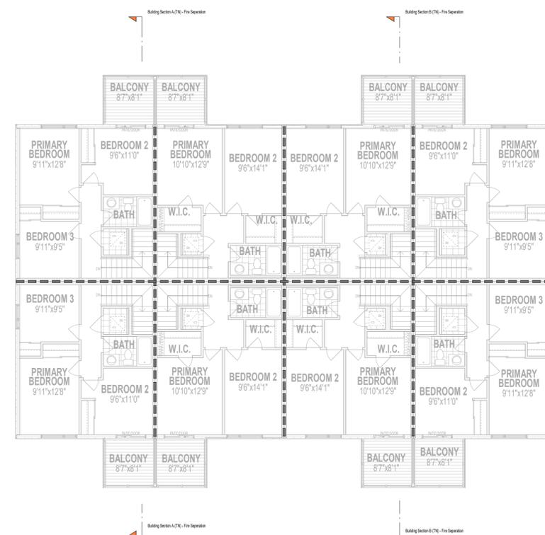
**THIRD FLOOR PLAN - FIRE SEPERATION PLAN**
