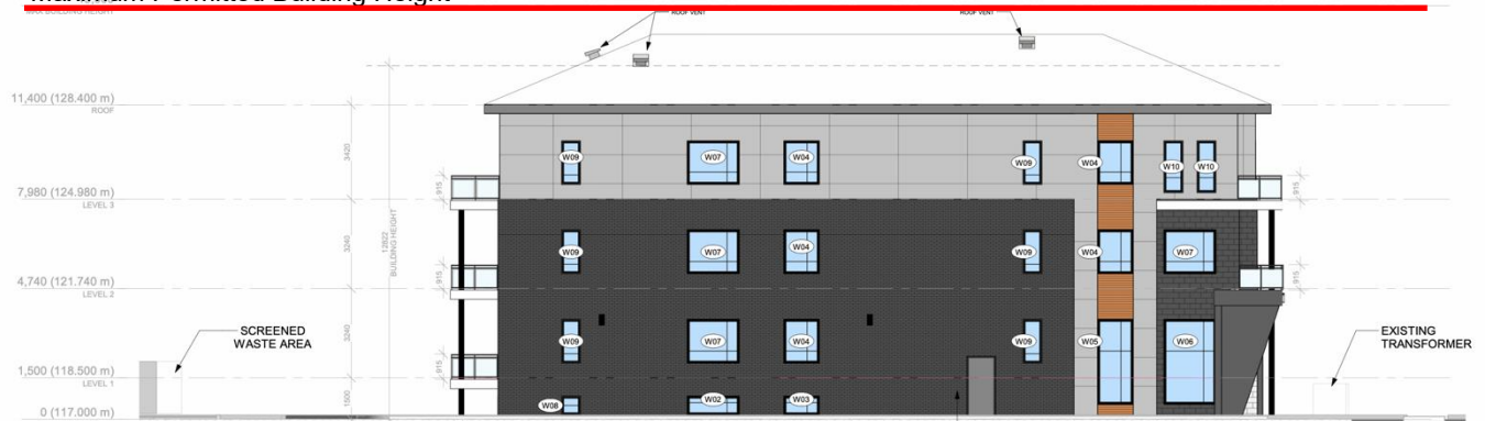
Figure 18: Elevation showing proposed building height compared to permitted building height.
