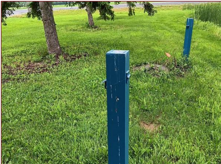
Photograph L1 – Looking west along the Dunning Road. View of two monitoring wells and a small ditch along Dunning Road..
