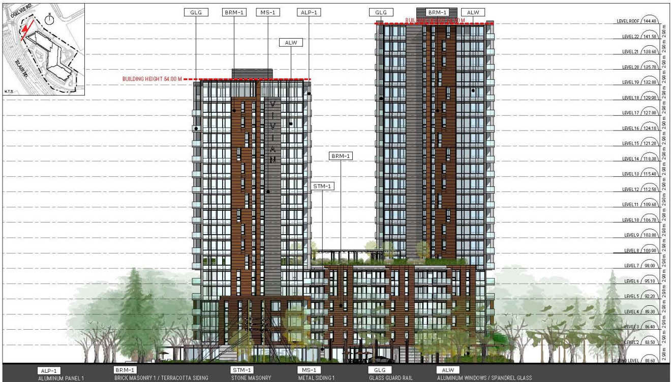
Figure 13: North Elevation. (Source: Hobin Architecture)
