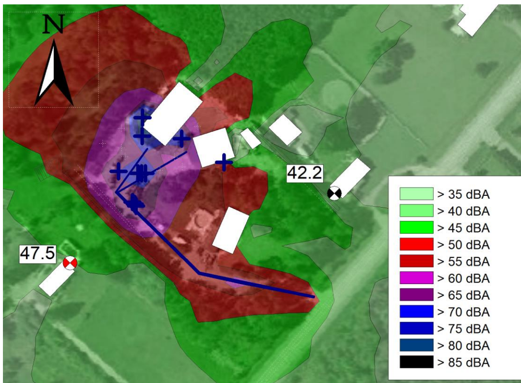
Figure 3.1 – Predicted sound pressure levels for existing conditions, as detailed in Section 2.3 . Sound pressure levels (SPL) for PORs in dBA. The grid was measured at 1.5m.
