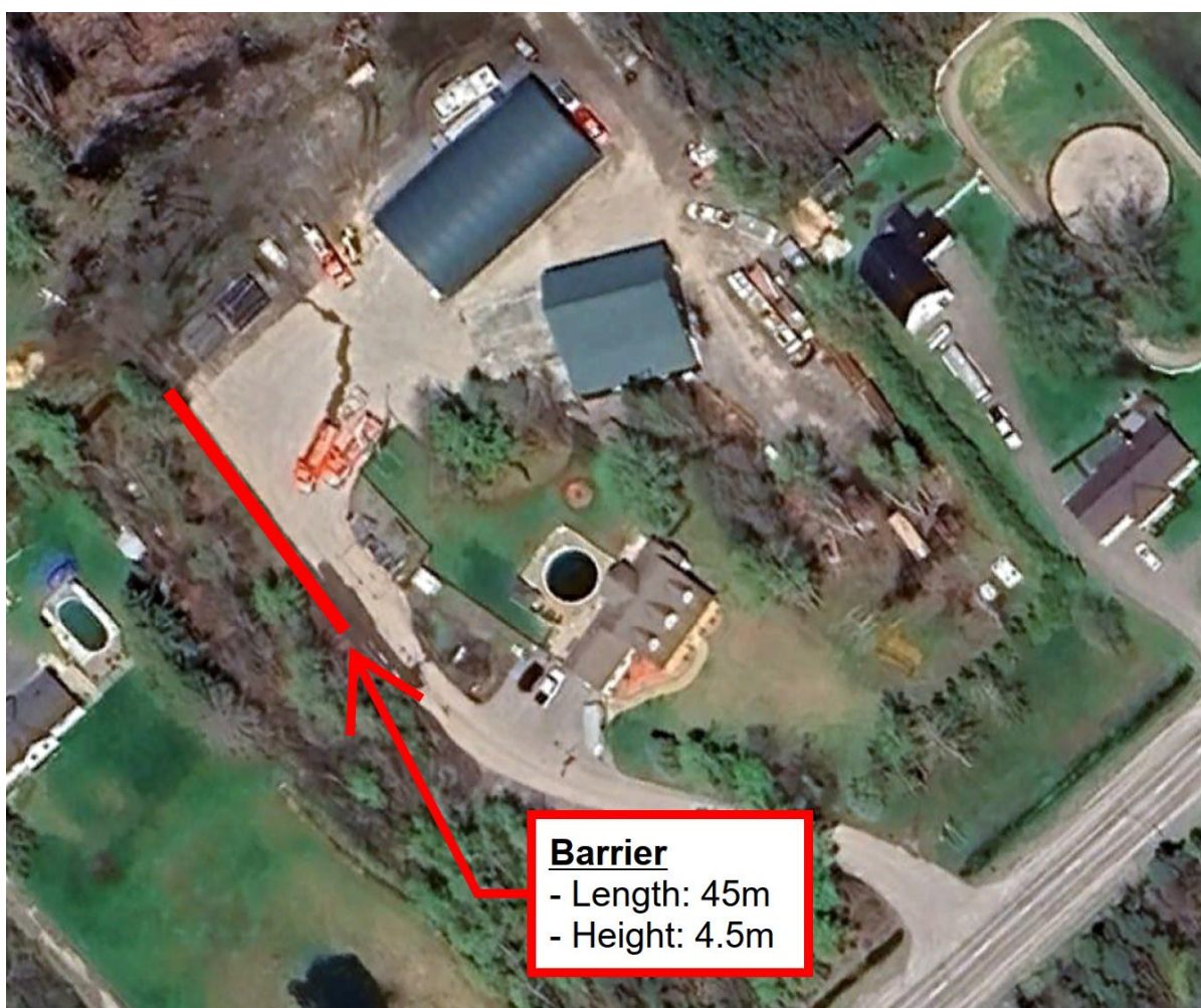
Figure 4.1 – Recommended approximate location and properties for the new barrier at Air Rock Drilling Headquarters (Satellite image from Google Earth Pro).
