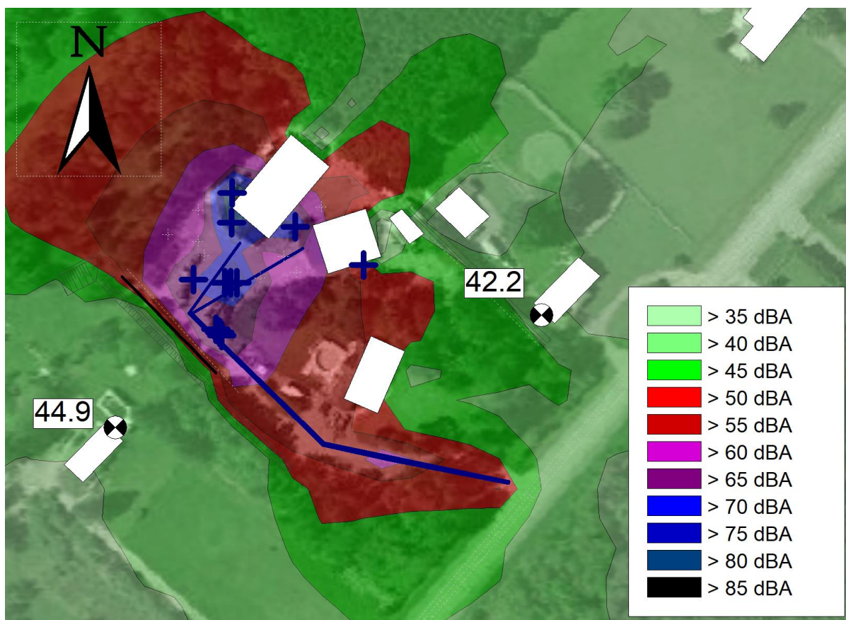
Figure 3.2 – Predicted sound pressure levels for existing conditions, as detailed in Section 2.3 , with acoustic mitigation. Sound pressure levels (SPL) for PORs in dBA. The grid was measured at 1.5m.
