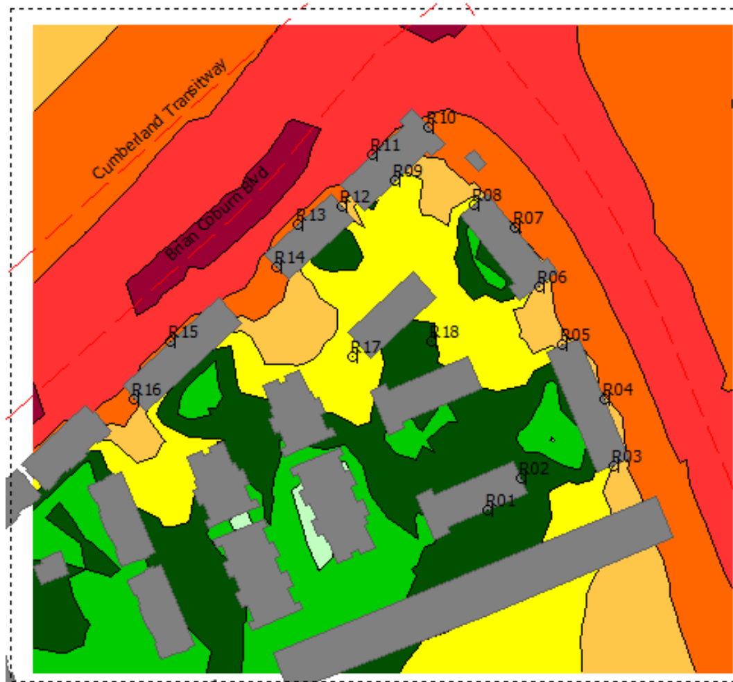
FIGURE 7: NIGHTTIME NOISE CONTOURS (4.5 M ABOVE GRADE)
