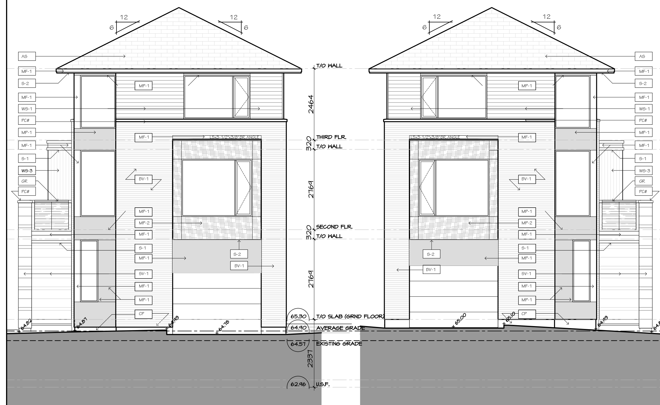
3 BLOCK T9 - SOUTH-EAST ELEVATION A2.09 SCALE 1:75
