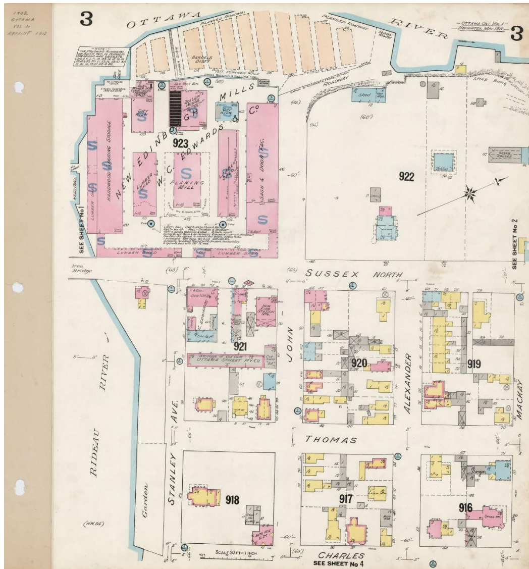
Figure 15: A portion of the 1901 revised 1912 Fire Insurance Plan indicates the primary building types in yellow are wood followed by brick veneer (pink outline & yellow) The masonry construction of the Allen House is in blue and solid pink indicates brick construction. . The lots such as 96 in the northern section of the village are larger with the two structures fronting MacKay on the same lot. The narrower lots south of Union Street dictated sideyard separation distance between buildings, with narrow frontage and buildings extending into the deep lots. The series of mid-block laneways providing access to the rear of the property are not found in the northern section of the district off Sussex. Source: Library and Archives Ottawa
