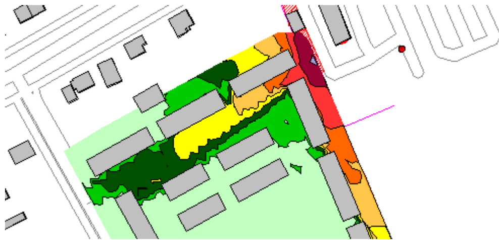
FIGURE 9: DAYTIME STATIONARY NOISE CONTOURS (1.5 M ABOVE GRADE)
