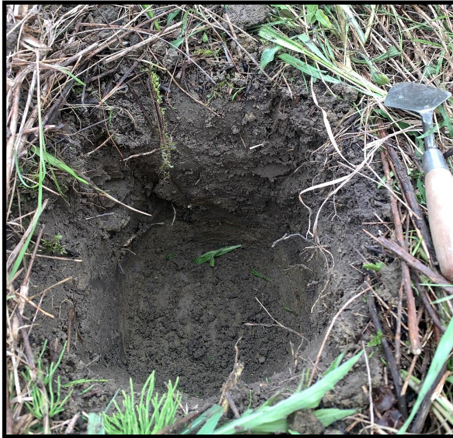
Figure 7: Typical test pit with greyish brown clay loam over greyish yellow clay subsoil. Southwest end of Parcel 4. (PA1148-D36)
