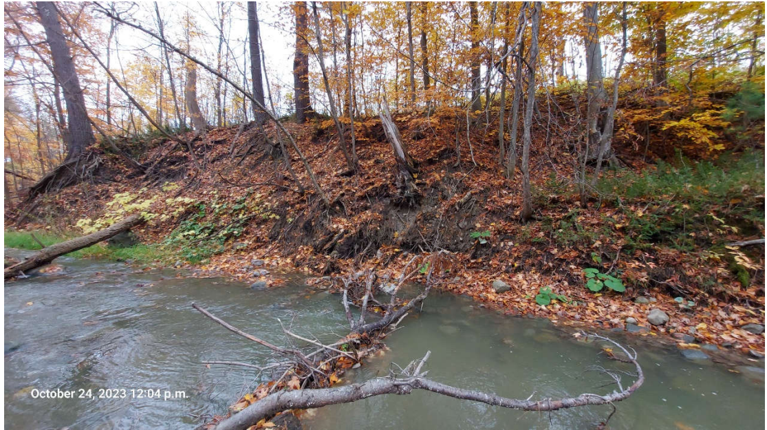
Photograph taken facing west along the right bank of the reach. Valley wall contact was observed at 3 occurrences throughout the reach, exposing tree roots and soil.
