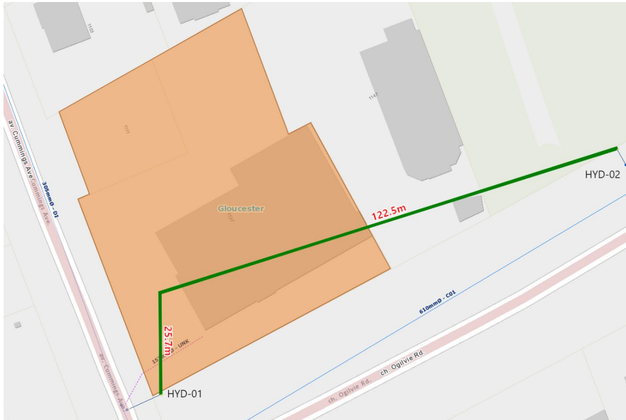
Figure 3-1: Existing Fire Hydrant Coverage Map
