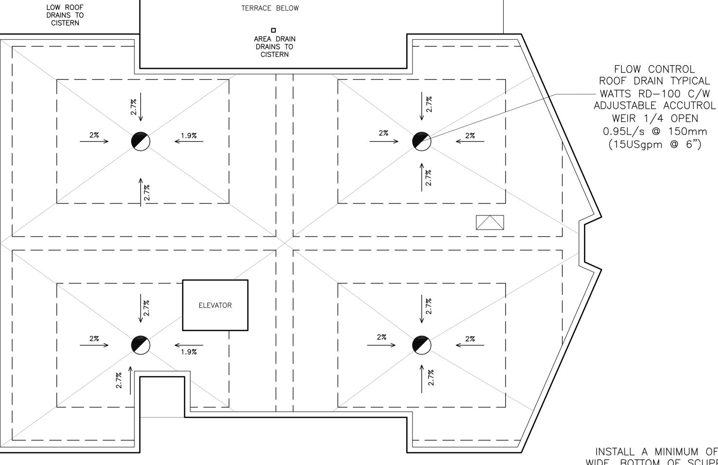
100 YEAR POND DEPTH AT ROOF DRAINS: 138mm
