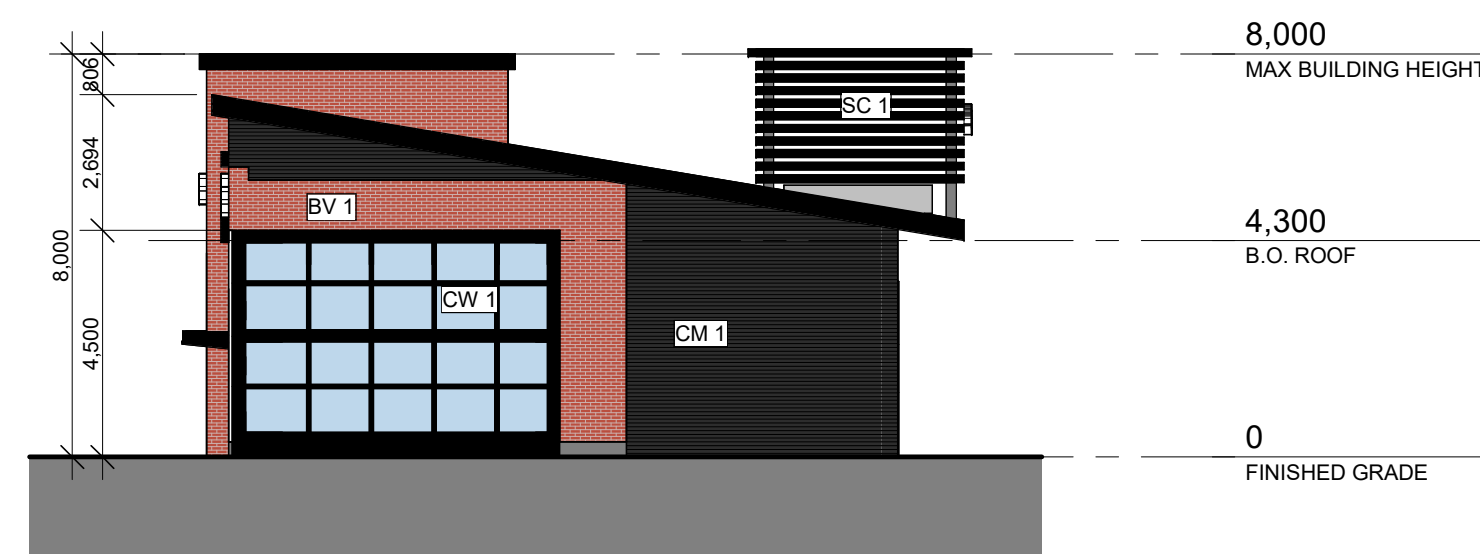
2 BUILDING B - EAST ELEVATION 1 : 150
