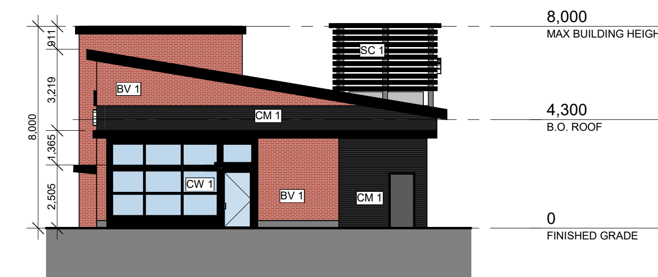
3 BUILDING F - WEST ELEVATION 1:150
