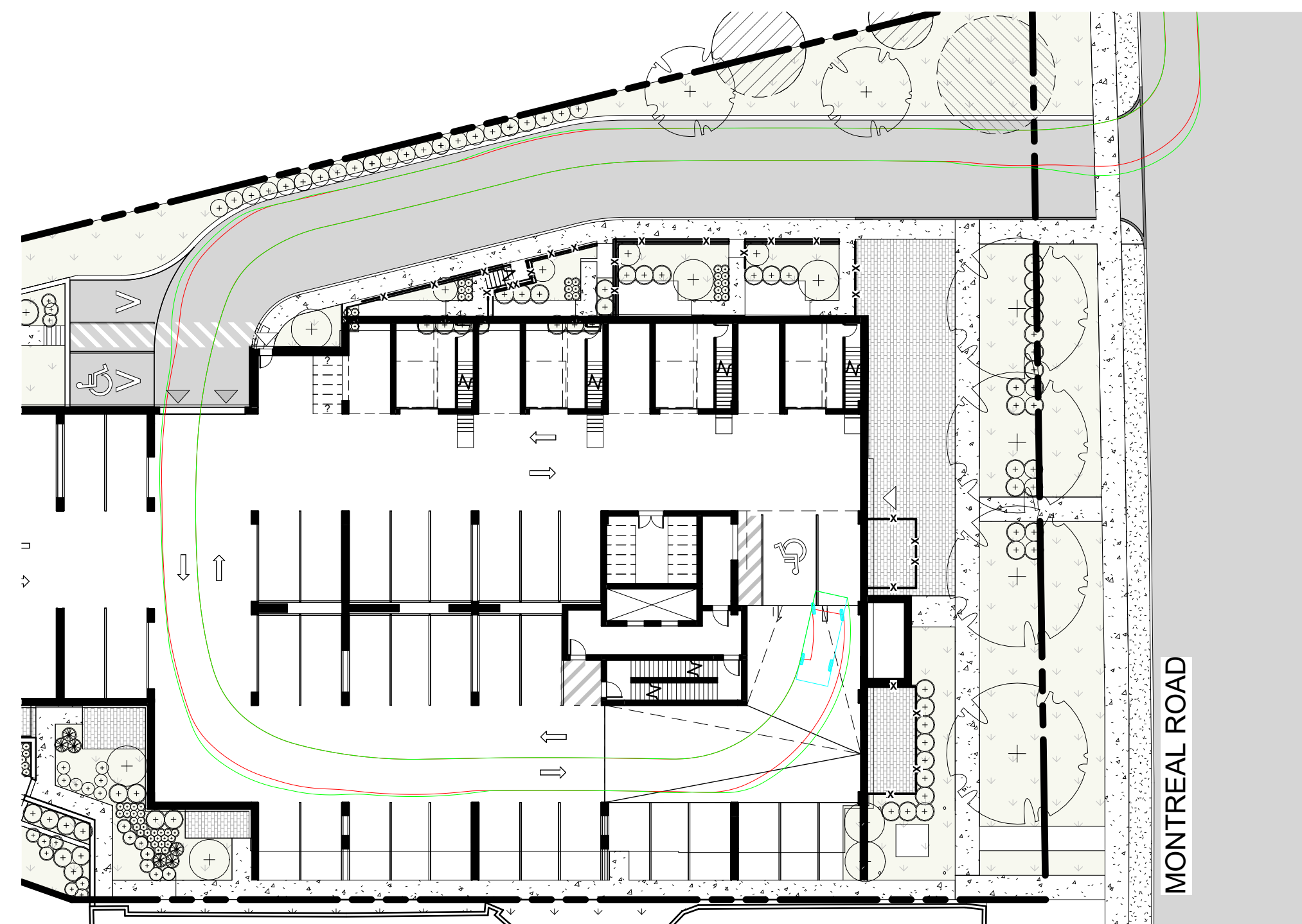
1 TURNING TEMPLATE - Car Entering A102 | 1:300
